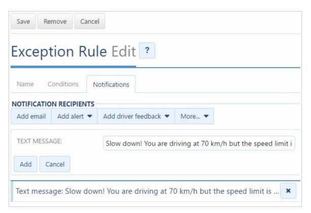
Once a driver triggers a rule, the Fleet Management Application will automatically send a message to the driver's message box in the Drive App.
